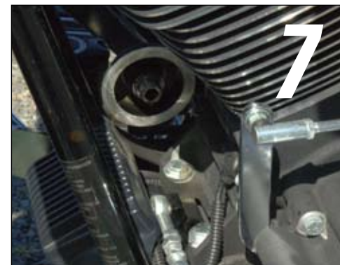
7. No mess! Reinstall oil pan plug, spin on and tighten a new filter wiping the rubber seal with fresh oil. Refill the crankcase. That's it!
