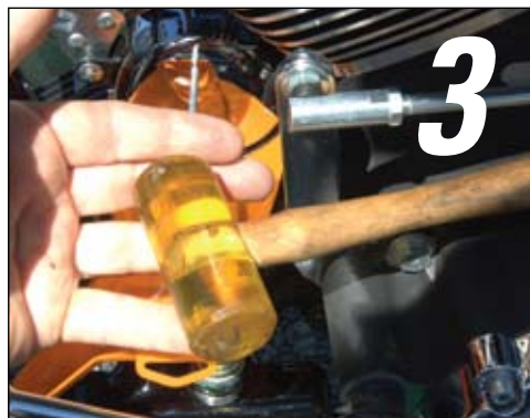
3. Punch a hole in top front of filter.
