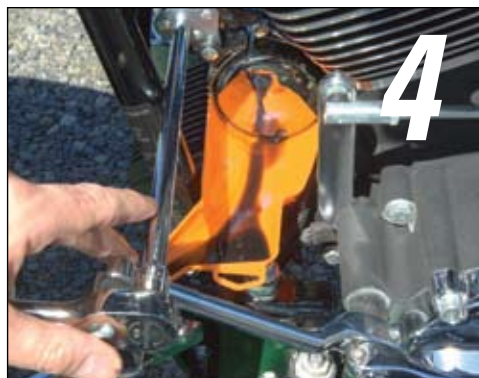
4. Twist oil filter off 1/2 turn until punched hole is at bottom. Do not break rear seal until oil is fully drained from filter.
