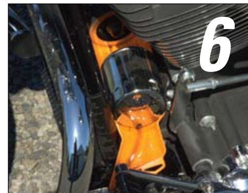
6. When filter is fully drained, spin off the rest of the way, into the filter funnel and remove oil filter and filter funnel together.
