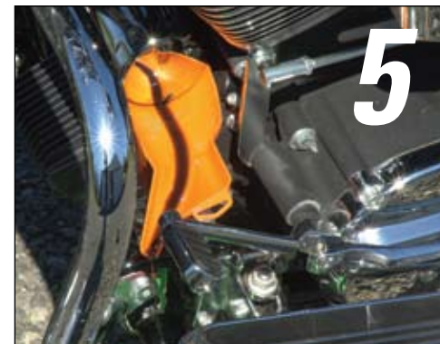
5. Remove oil drain-plug and dipstick. Let drain completely. Use tube provided to drain it away from chassis.
