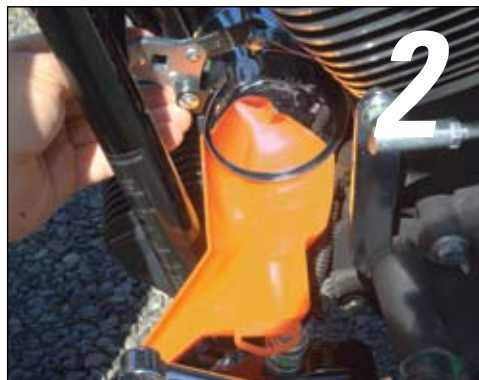
2. We used a clamp-type oil filter wrench for clearance.
