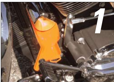
1. Place Greg's Oil Filter Funnel below the oil filter.
